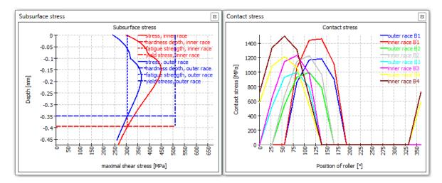
The load zone for the bearings is relatively small. It is only about 140°.
