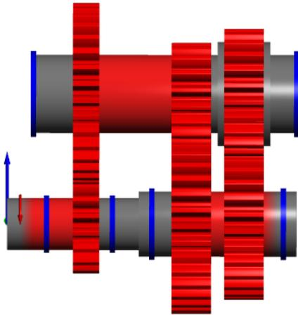
The power will first flow through the gear pair 'C in-C out', whose gears are constantly engaged, and will be eventually transmitted through the gear pair 'G1 in-G1 out', so we will set the flag of the corresponding check box.
