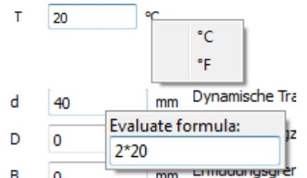
Pressing the right mouse button on an input field a window for an input of a formula is shown. This can be used for quick calculations.
