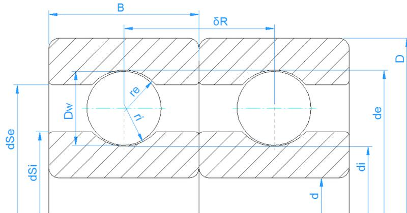
The geometry data is defined for a single deep groove ball bearing, additionally the distance between the two rows is an input value. The input of the diametral clearance is for the single bearing only.
