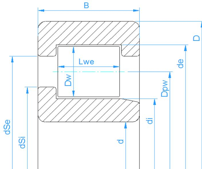
The roller profile is considered as defined by ISO/TS 16281 as default. If the extended calculation for pressure distribution is selected an input of profile for races and roller is possible using the  $\oplus$ -button behind the roller effective length. Several options are available including reading the profile from a file.
