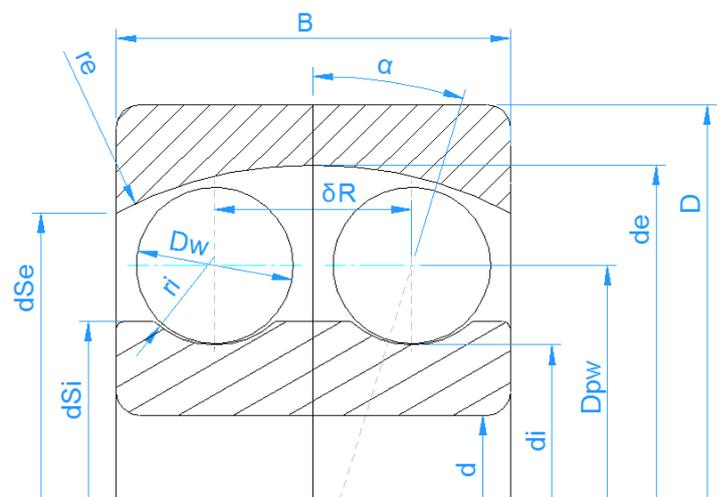
The shoulder diameter of the outer ring is automatically limited by the width and the radius of the outer race. Still a larger value as the limit could be entered by the user. The life modification factor  $a_{ISO}$  is calculated for both rows separately.
