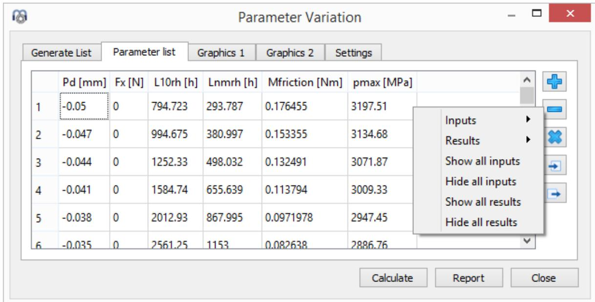
By clicking on 'Calculate' while the "Generate list" tab window is active, a list of all parameter combinations will be generated at the corresponding tab window 'Parameter list' and the analysis will be run. Depending on the chosen number of parameters and steps, the analysis can lead to long calculation times.
