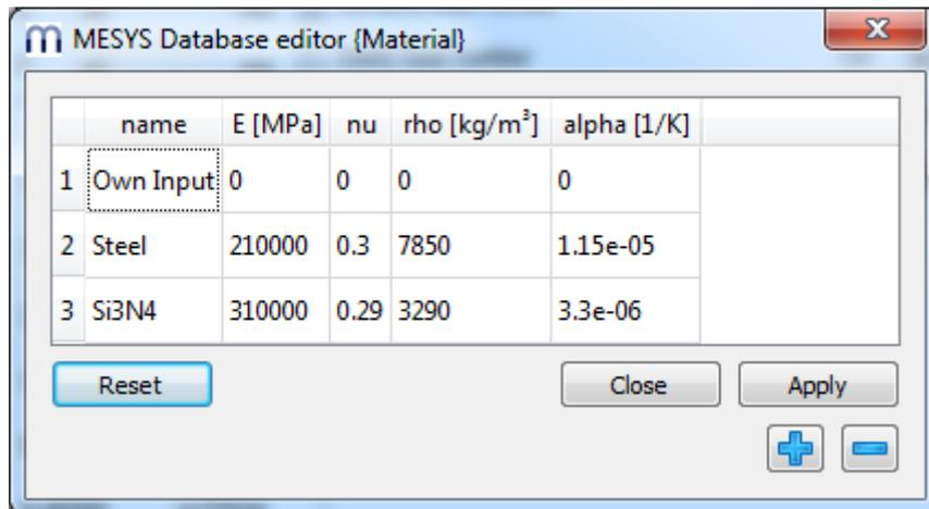
Data is written into the database only when clicking the Apply-Button, changes can be removed by selecting 'Reset' before 'Apply' is clicked.
