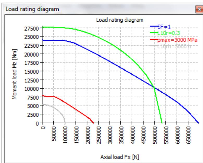
For each axial load the tilting moment is increased until the selected criteria are reached. The number of points used for one line and a tolerance for the calculation can be defined.
