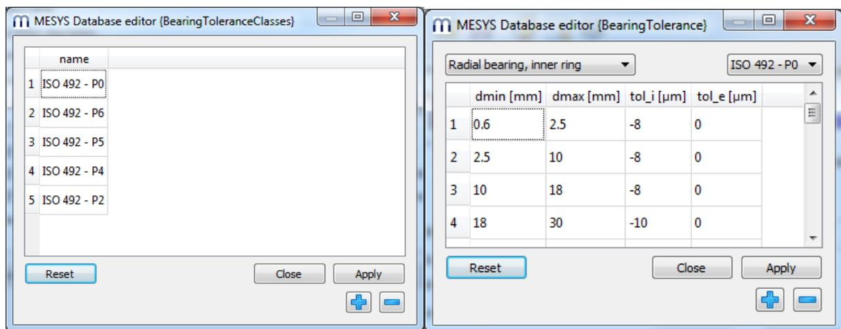
In table ‘BearingClearance’ and ‘BearingTolerance’ then the actual values are defined dependent on the diameter.
