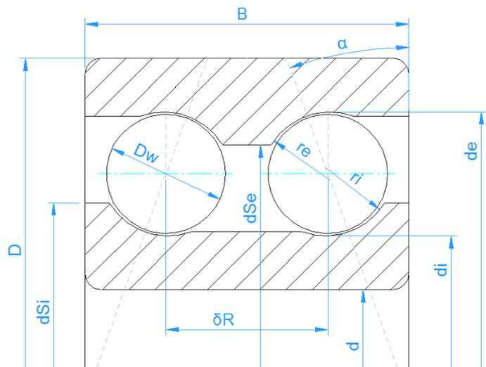
In addition to the inputs for the single row angular contact bearing the distance between rows has to be entered.
