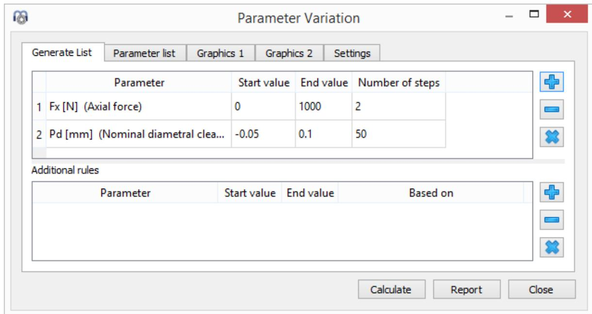
Additional rules can be used to set additional input parameters dependent on parameters on the first list. The additional parameter is interpolated between a start and end value based on another parameter. For example additional parameter y between y1 and y2 based on parameter x in range x1 to x2:
