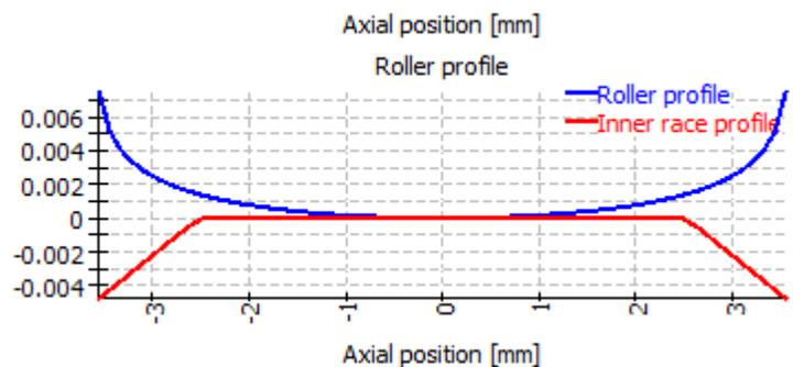
The unsymmetrical profile is used from left to right for most bearings. For taper roller bearings and axial spherical roller bearings the profiles is used from left to right if direction of contact angle is left. For contact angle to the right the profile is mirrored. So mounting conditions do not influence the profile.
