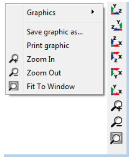
In the graphic windows of the software, there are different buttons for the view manipulation in 3D, such as the zoom-in, zoom-out and fit-to-window functions and also it is possible to select the point of view from different planes. The 3D model can be dragged with the mouse by holding down SHIFT key as well as zoomed in and out by holding down the CTRL key.
